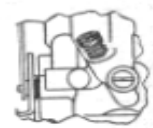
Idle Adjustment Screw Setting 1/2 to 1 Turn Open
